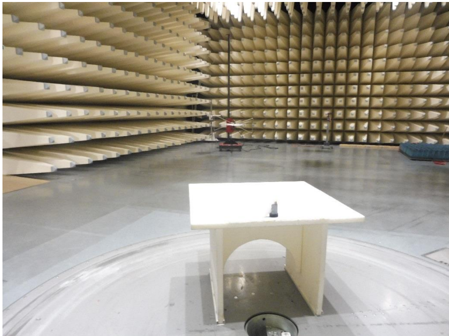
Photo 12: EUT at the semi-anechoic chamber
