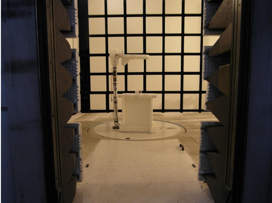
Photo 7: EUT at the anechoic chamber, loop antenna test setup at 80 cm height
