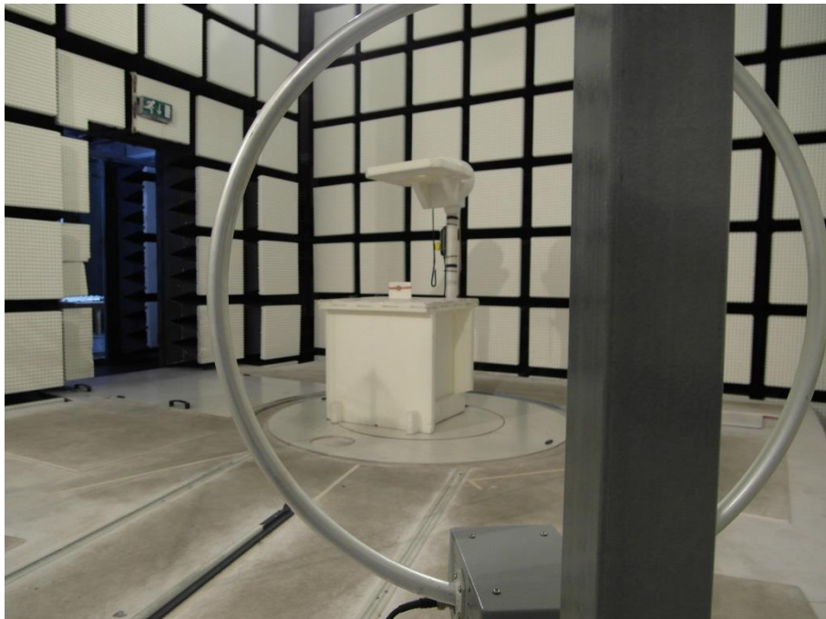
Photo 10: EUT at the anechoic chamber, loop antenna test setup at 80 cm height
