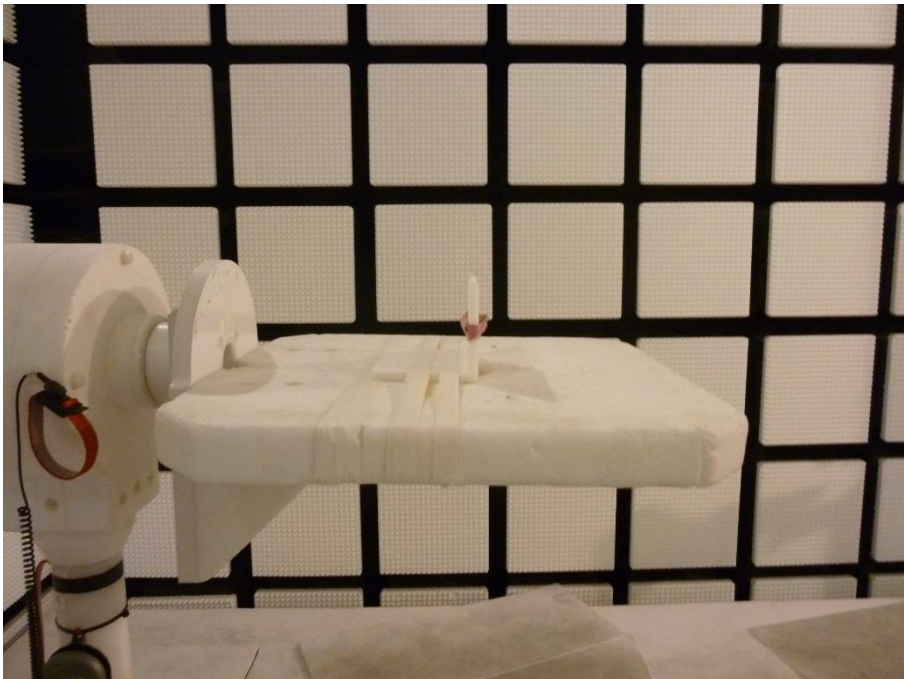
Photo 2: EUT at the anechoic chamber
