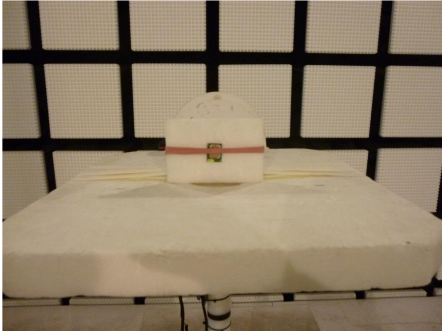
Photo 5: EUT at the anechoic chamber
