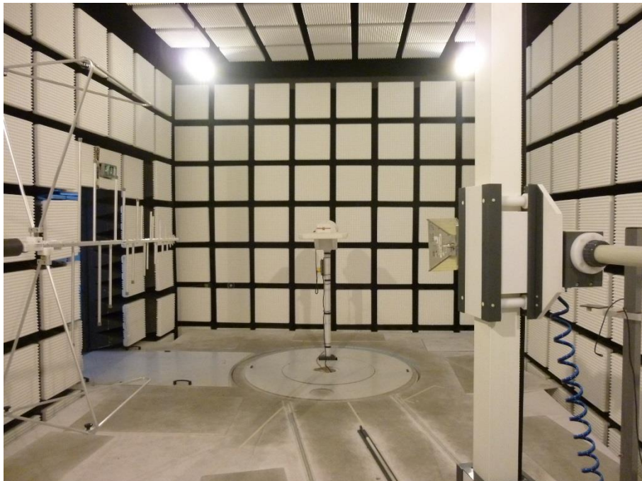
Photo 6: EUT at the anechoic chamber
