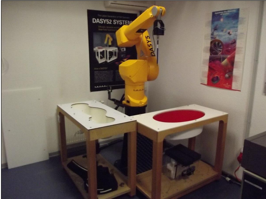
Photo 1: Measurement System DASY 5
