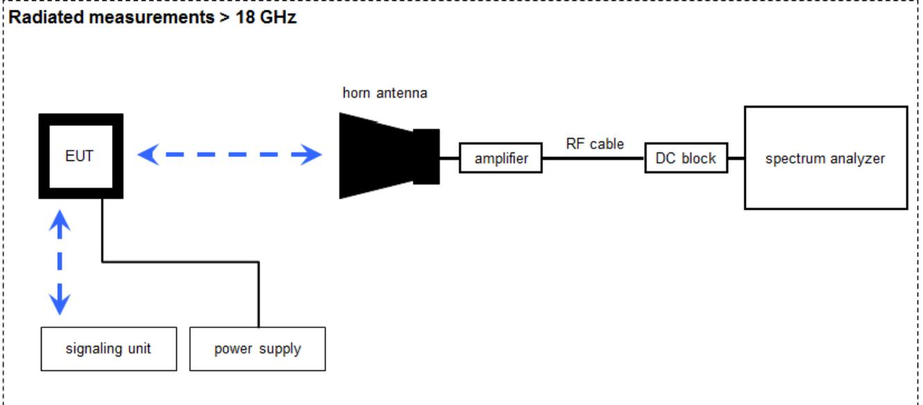
Measurement distance: horn antenna 50 cm
