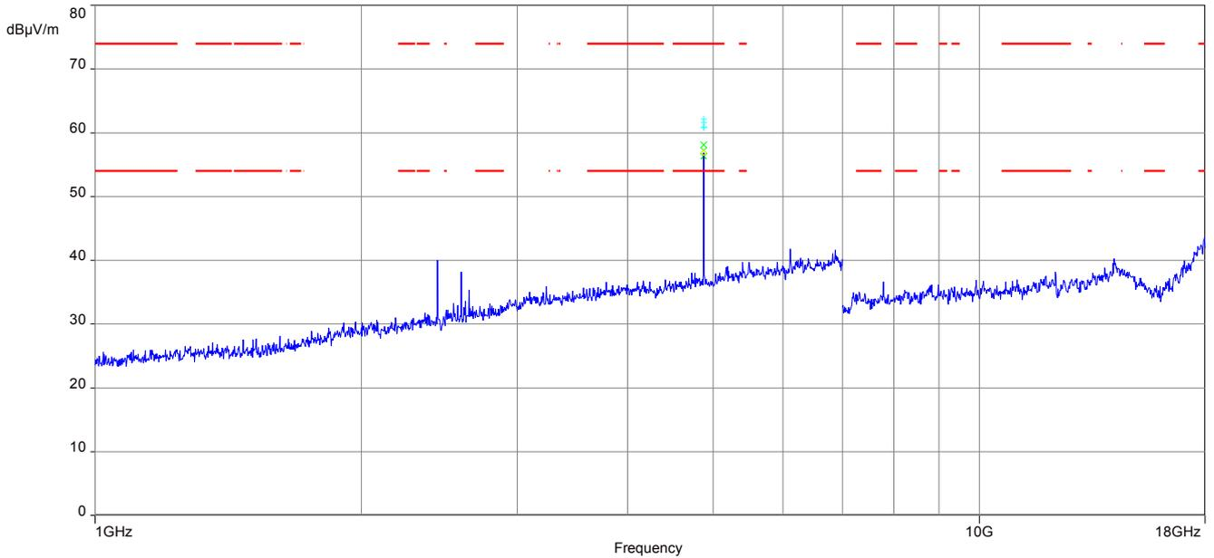
The carrier signal is notched with a 2.4 GHz band rejection filter.
