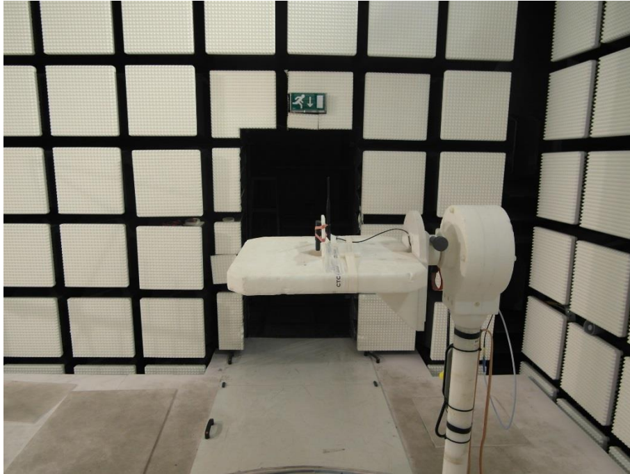
Photo 3: EUT at the anechoic chamber
