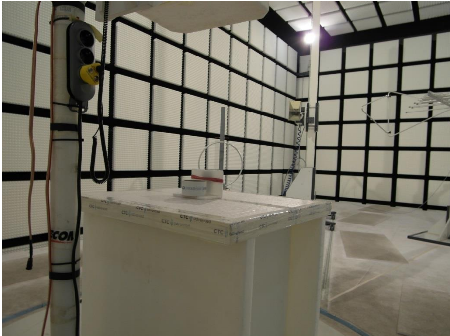
Photo 8: EUT at the anechoic chamber, loop antenna test setup at 80 cm height
