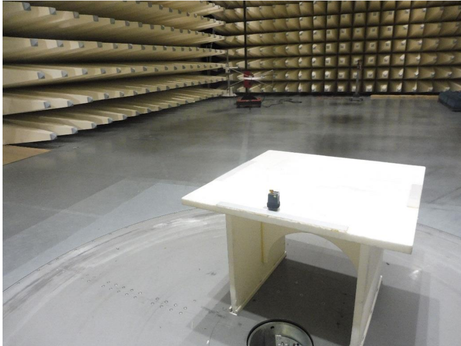
Photo 11: EUT at the semi-anechoic chamber
