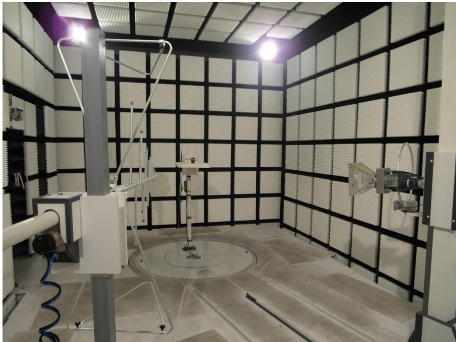
Photo 6: EUT at the anechoic chamber
