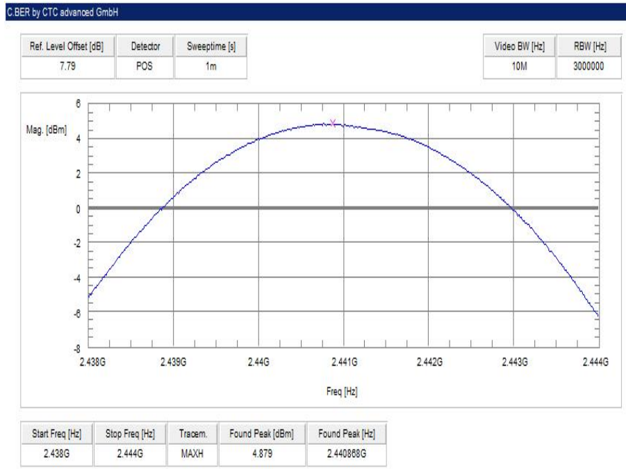
Plot 5: middle channel – 2441 MHz, Pi / DQPSK modulation
