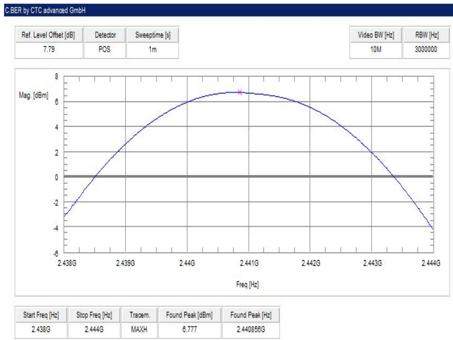
Plot 2: middle channel – 2441 MHz, GFSK modulation
