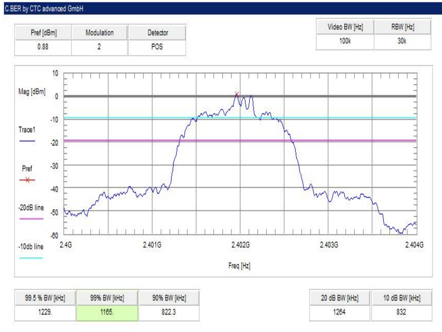
Plot 7: lowest channel – 2402 MHz, 8 DPSK modulation
