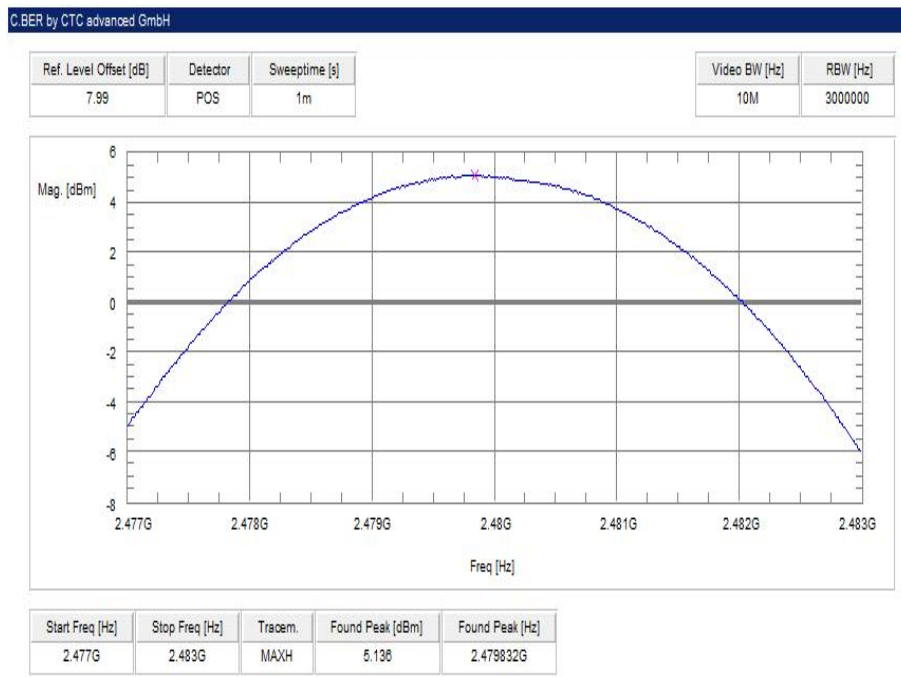
Plot 6: highest channel – 2480 MHz, Pi / DQPSK modulation
