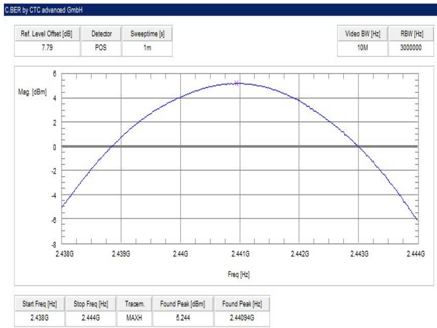
Plot 8: middle channel – 2441 MHz, 8 DPSK modulation
