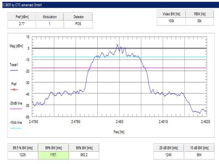
Plot 6: highest channel – 2480 MHz, Pi / DQPSK modulation
