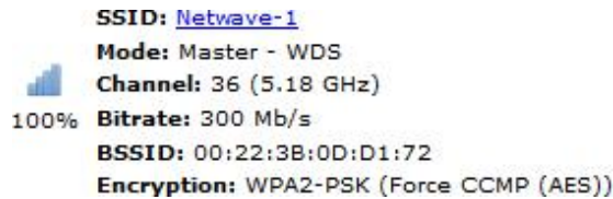
Figure 4: A summary in the Wireless section for a device operating as an 802.11 access point.
