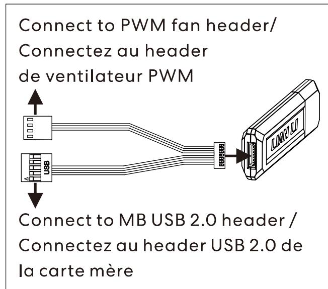
Each L-Wireless Controller supports 10 channel of device/
