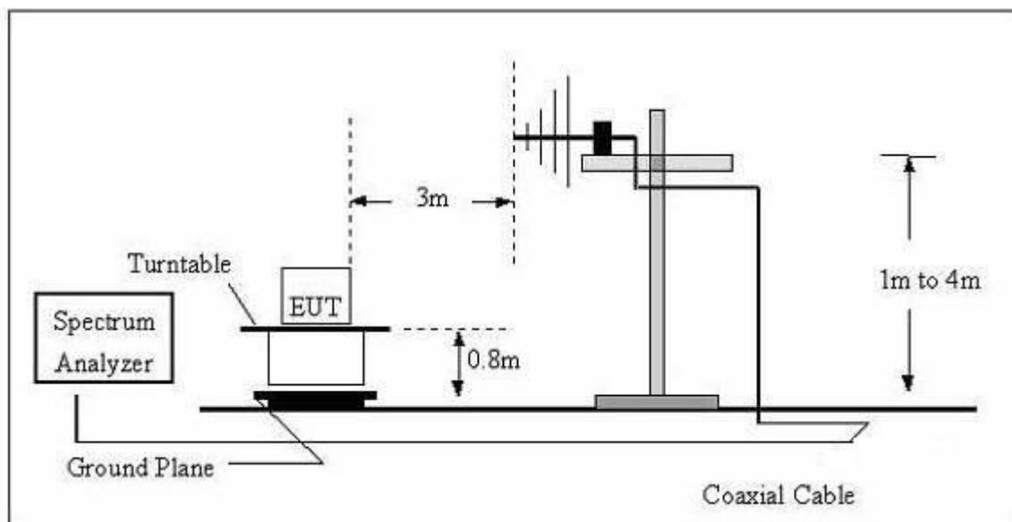
(C) For radiated emissions above 1000MHz
