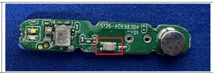
The antenna is Chip antenna. The best case gain of the antenna is 1.95dBi.
