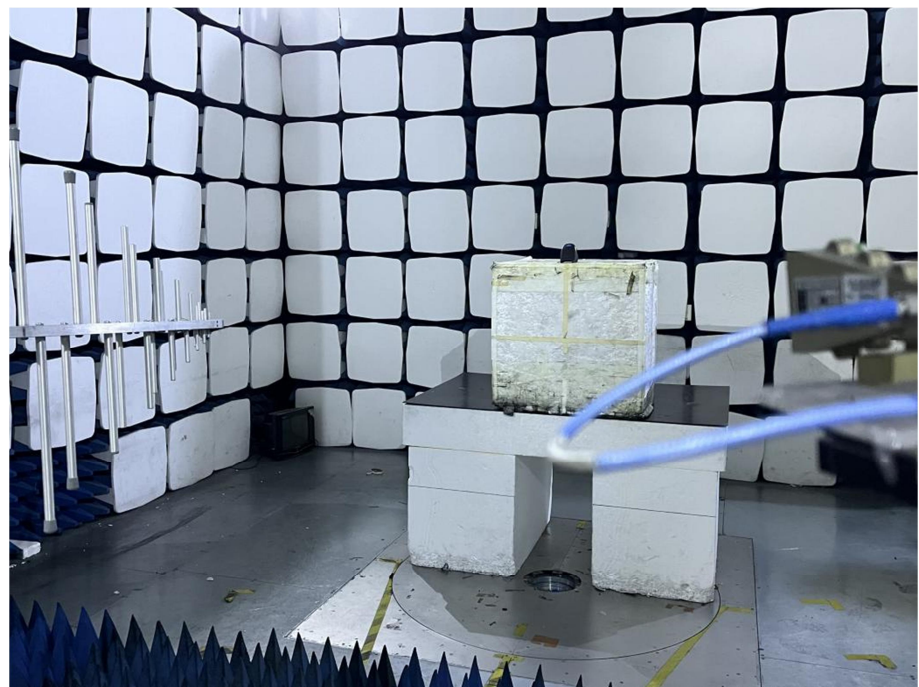
Radiation Emission Test Setup (Above 18GHz)
