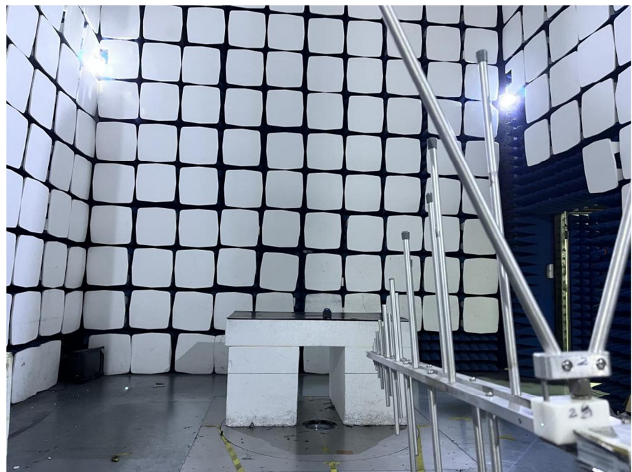
Radiation Emission Test Setup (30MHz to 1GHz)
