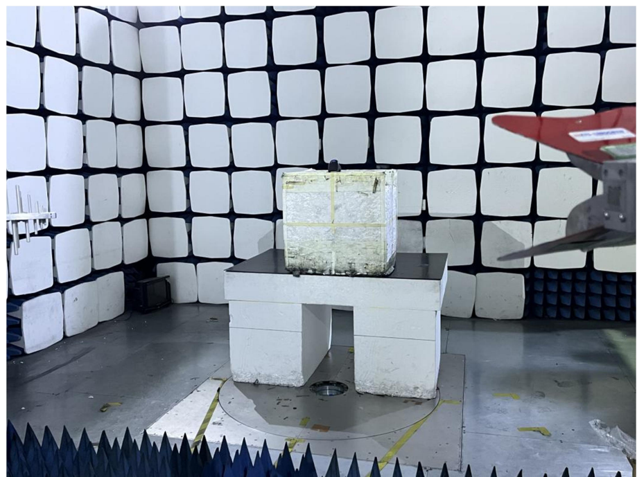
Radiation Emission Test Setup (1GHz to 18GHz)
