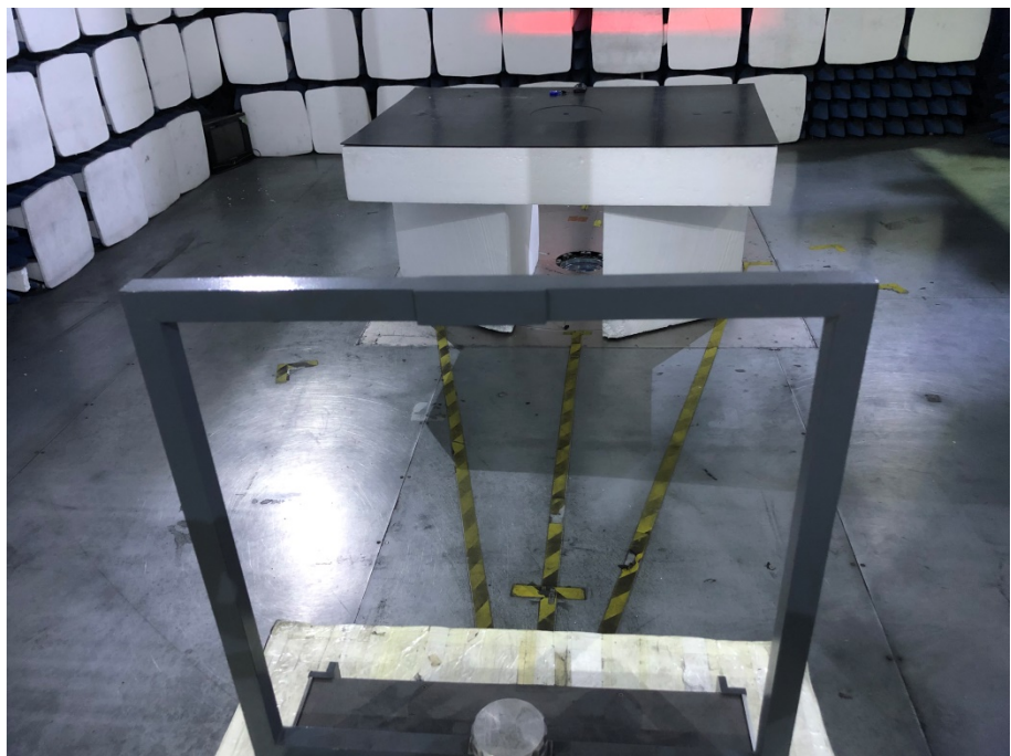
Radiation Emission Test Setup (Below 30MHz)
