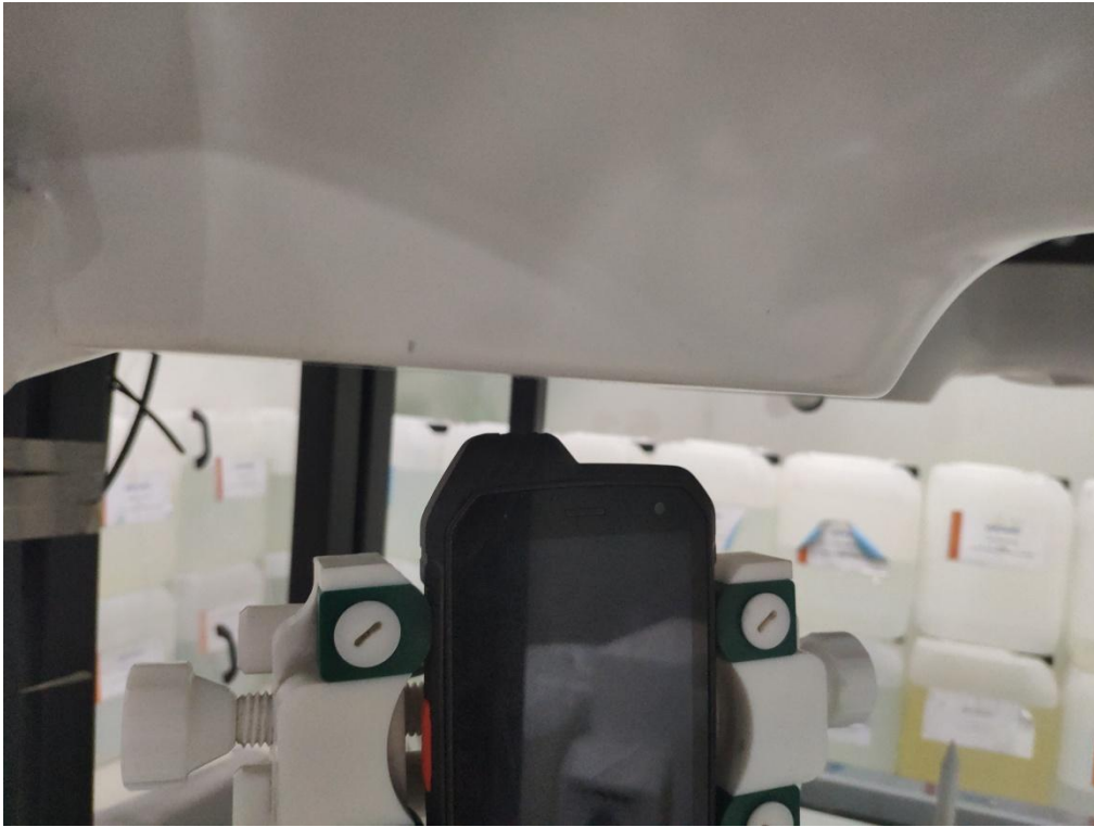
Body top side(separation distance is 10mm)
