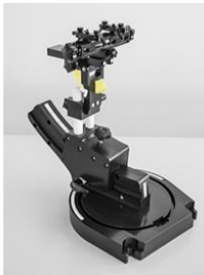
Device holder supplied by SPEAG
