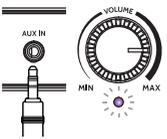
The 3.5mm AUX-IN port is ideal for playback of audio from older mobile devices without Bluetooth capability. Connect your device to the AUX-IN port (19) with a 3.5mm stereo jack lead (not supplied). Power on the turntable and the auxiliary device, the LED will light up purple. Adjust the volume on the N10, Use the controls of your auxiliary device for all other actions. Please Note: The AUX-IN function overrides all others no matter what the mode setting is.
