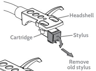
To fit a new stylus, slot it onto the cartridge, then lift and rotate the stylus until it clicks into place
