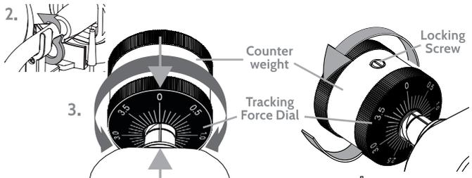
Unclip the tonearm position the tonearm in the space between the tonearm rest and the platter.
