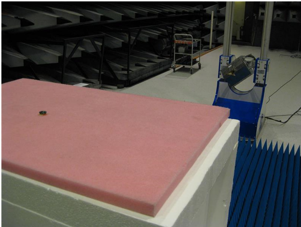
Photo 1.1.2 Test setup regarding measurement of band edge compliance.
