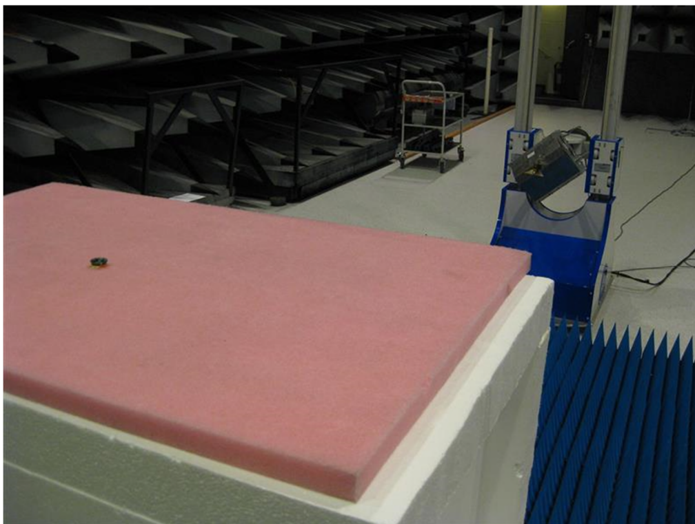
Photo 4.4.2 Test setup regarding measurement of radiated emission (above 1 GHz).
