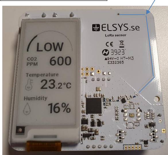
Front-side without PIR. No module. Models: ETHd10, EIAQd10
