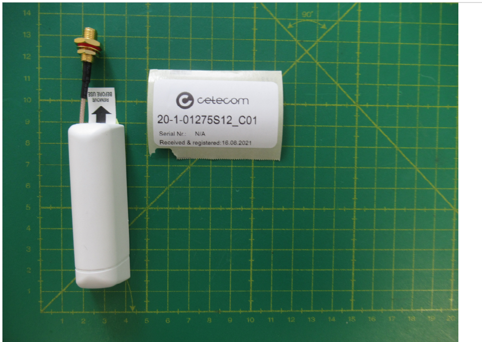
Photograph 3: EUT 2_conducted 125 kHz FHSS fixed channel_with case
