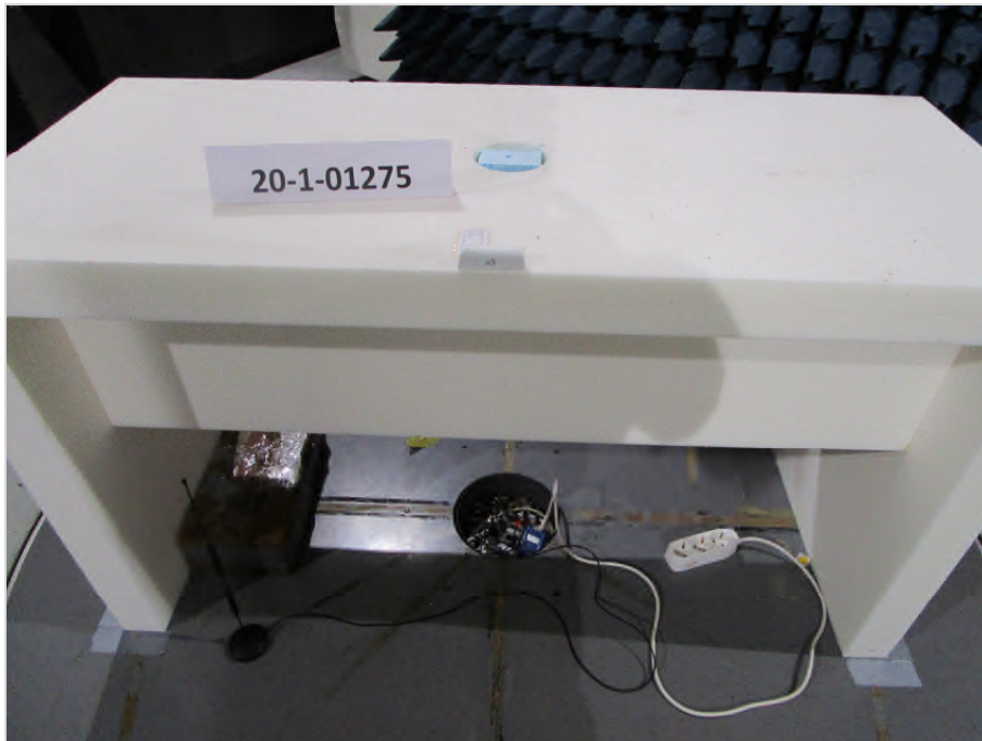
Photograph 1: Setup 1 in the semi anechoic chamber, Radiated interference field strength close up view
