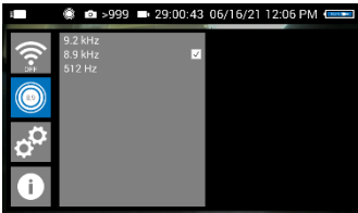
Fig. 32: Locator detection with 8.9 kHz transmission frequency selected
