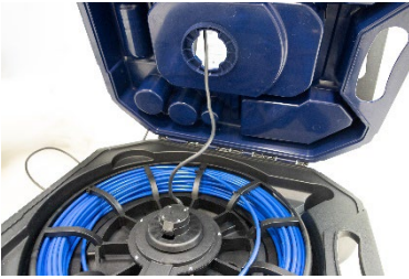
Fig. 60: Wrong: Camera cable not pulled tight
