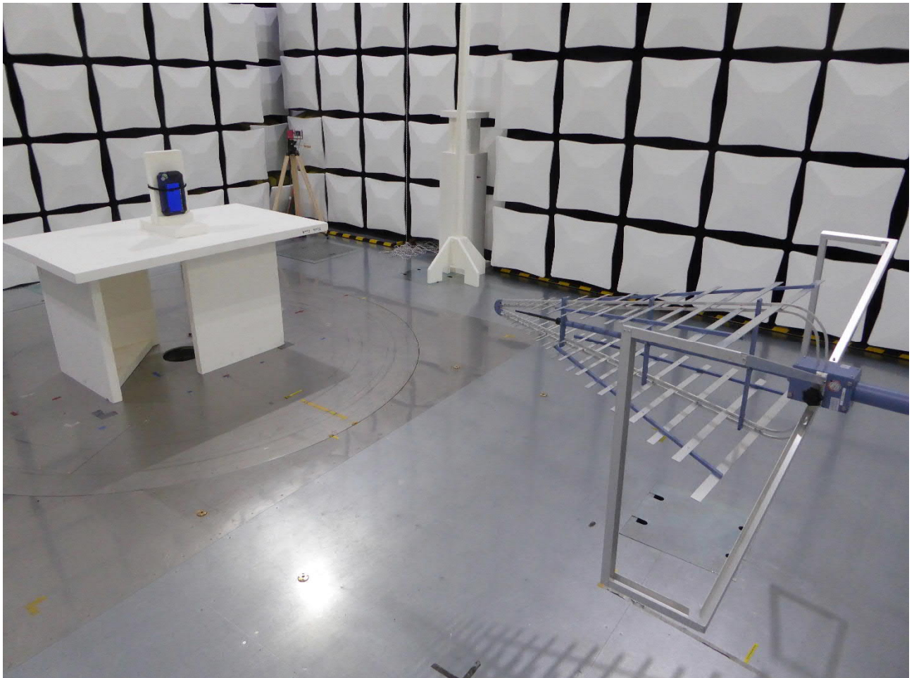
Test setup semi anechoic chamber 30 MHz – 1 GHz (Pos 3)
