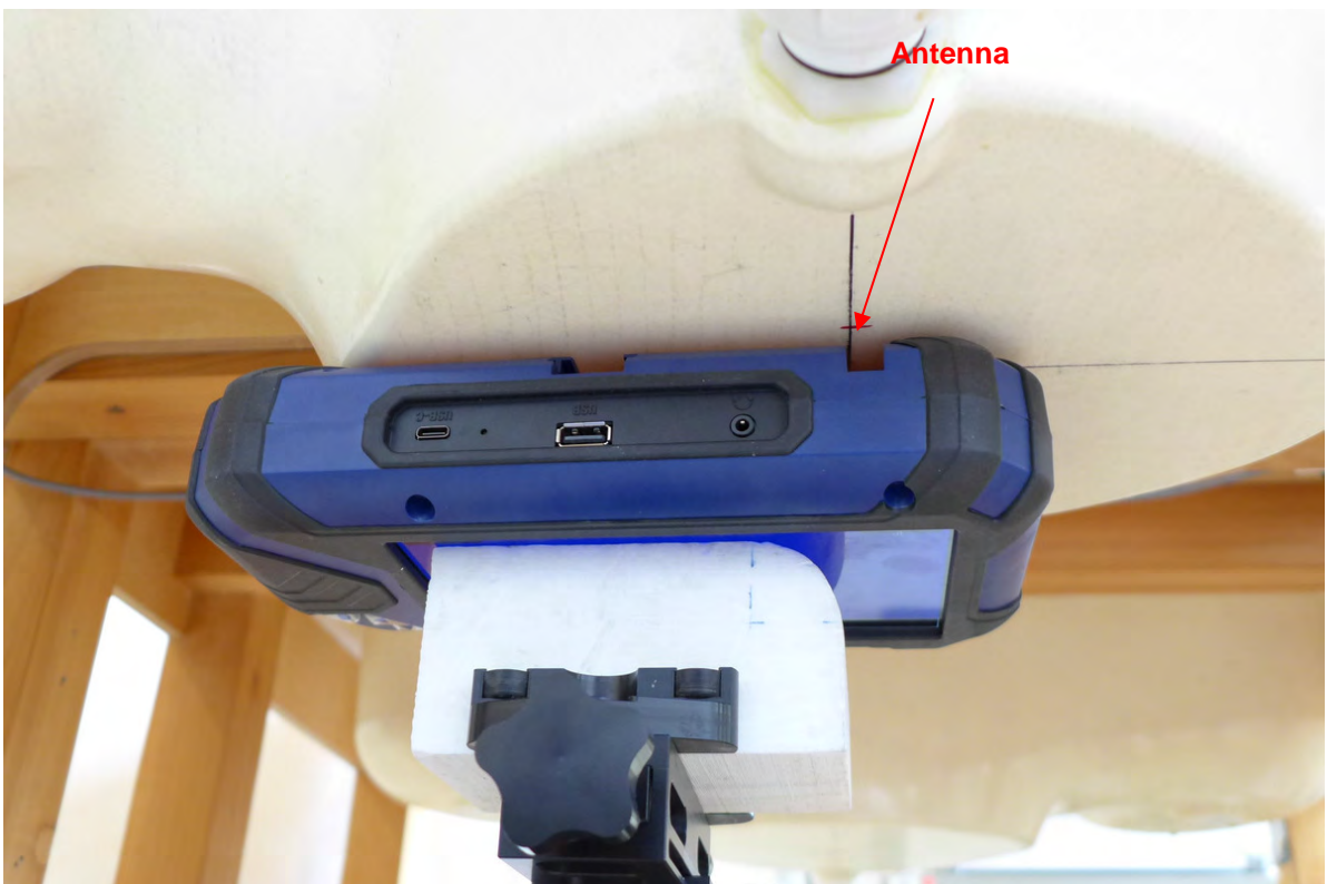
Pic. 5: Test position rear side of DUT towards the phantom, 0 mm gap.
