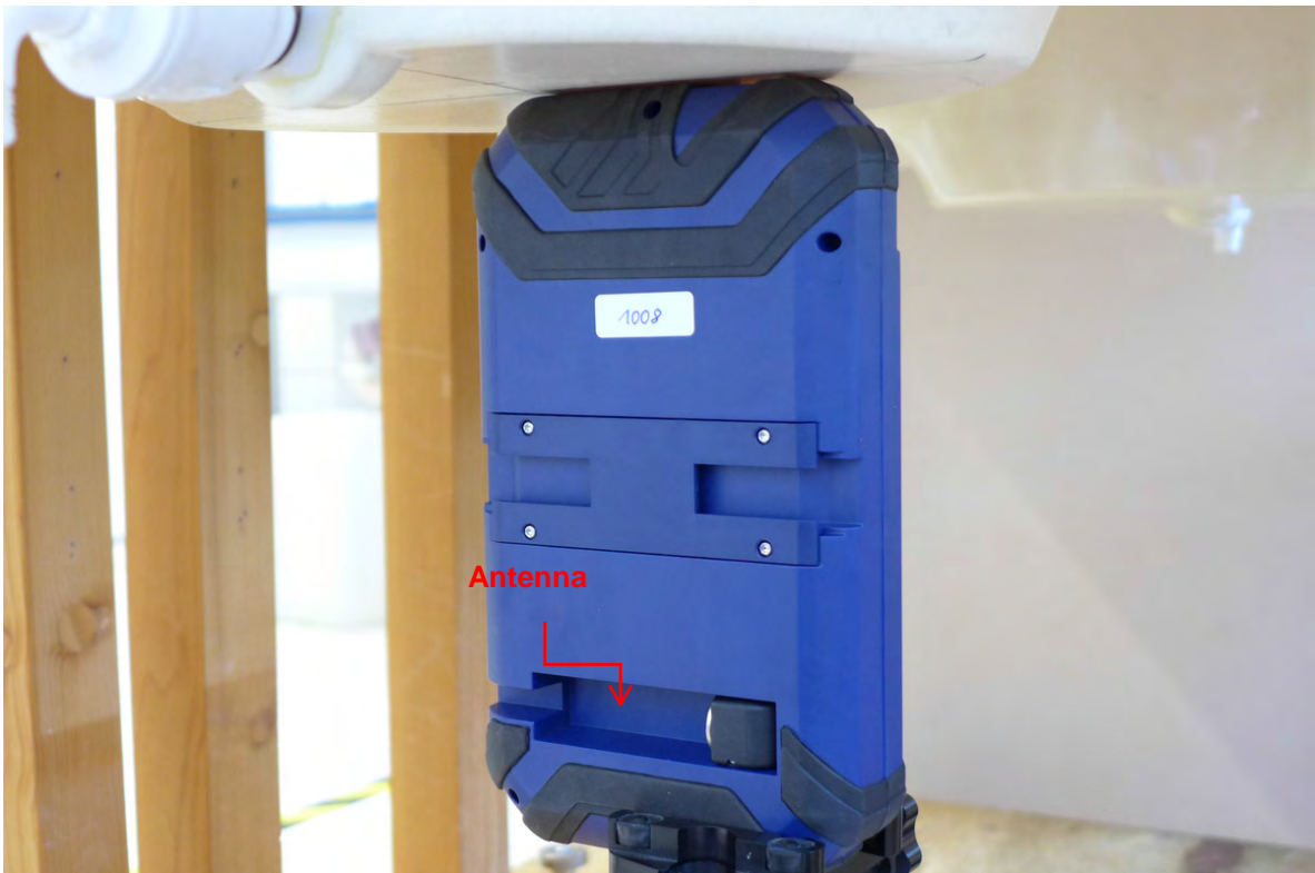
Pic. 7: Test position right side of DUT towards the phantom, 0 mm gap.
