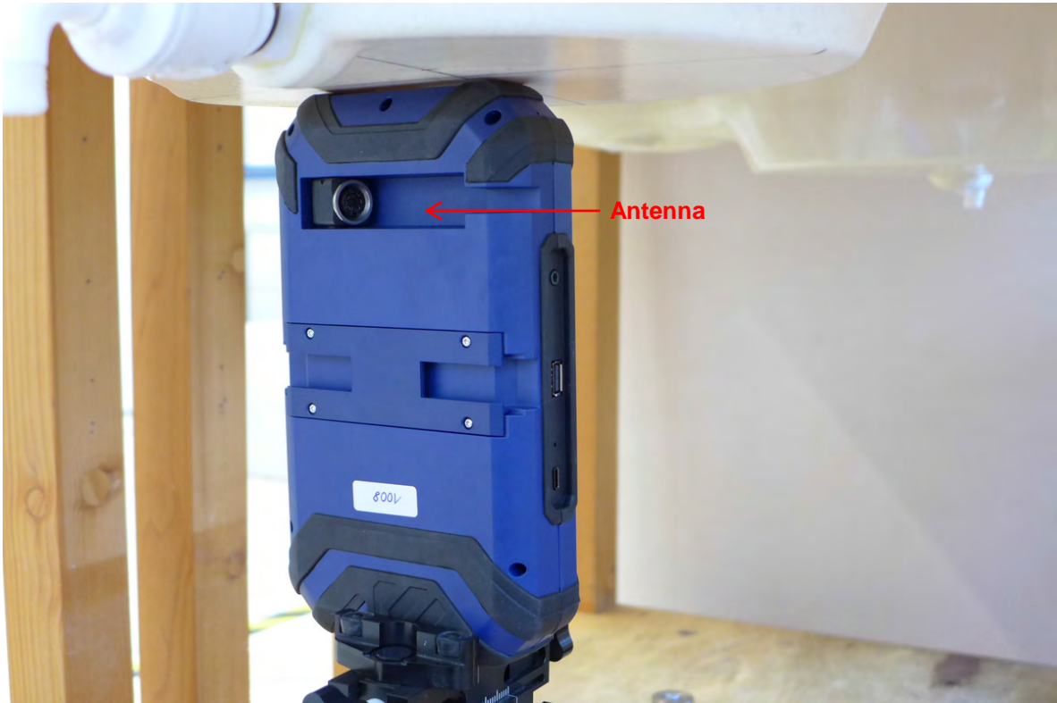
Pic. 6: Test position left side of DUT towards the phantom, 0 mm gap.
