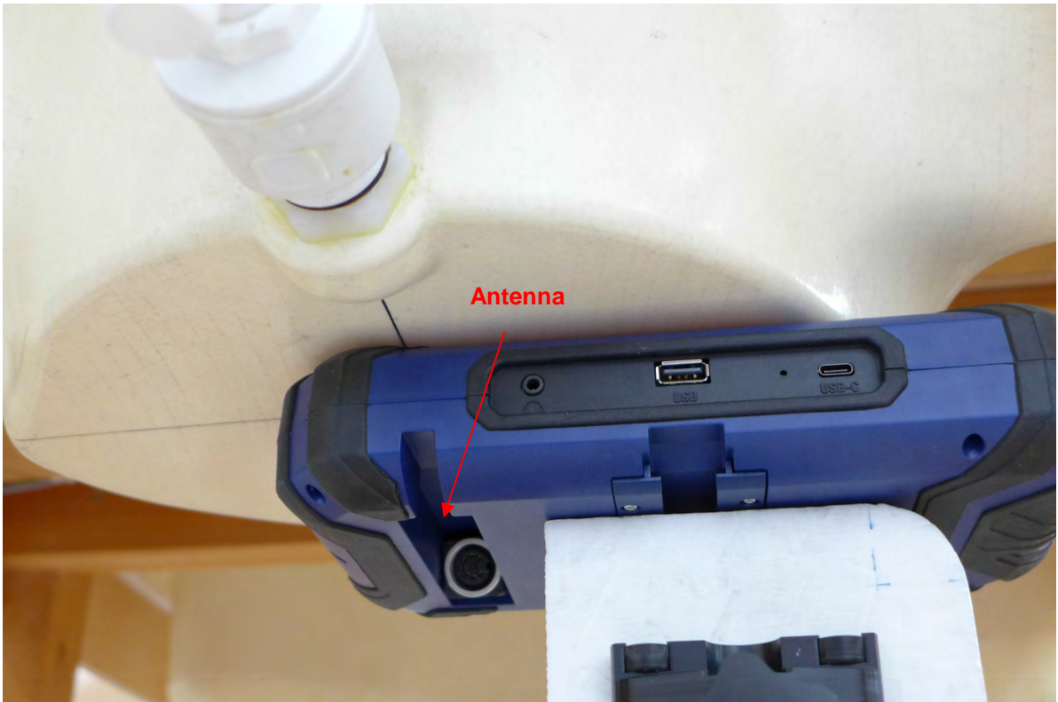
Pic. 4: Test position front side of DUT towards the phantom, 0 mm gap.
