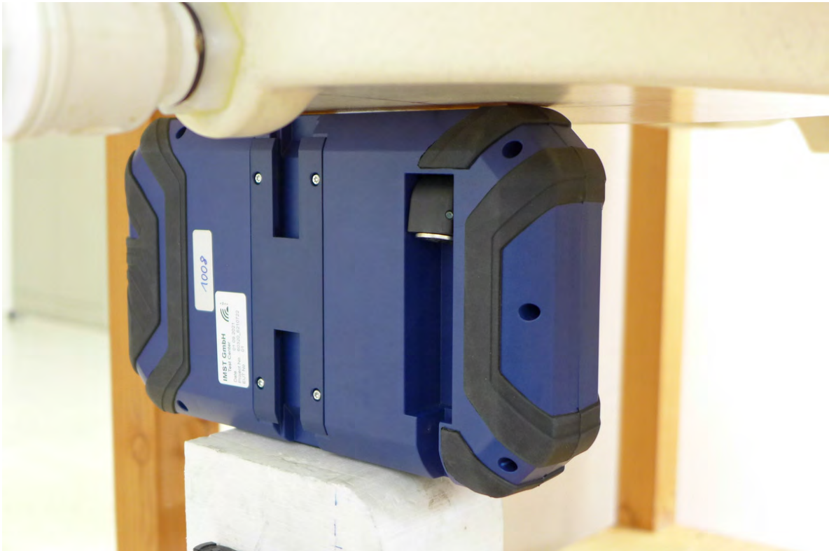
Pic. 8: Test position top side of DUT towards the phantom, 0 mm gap.
