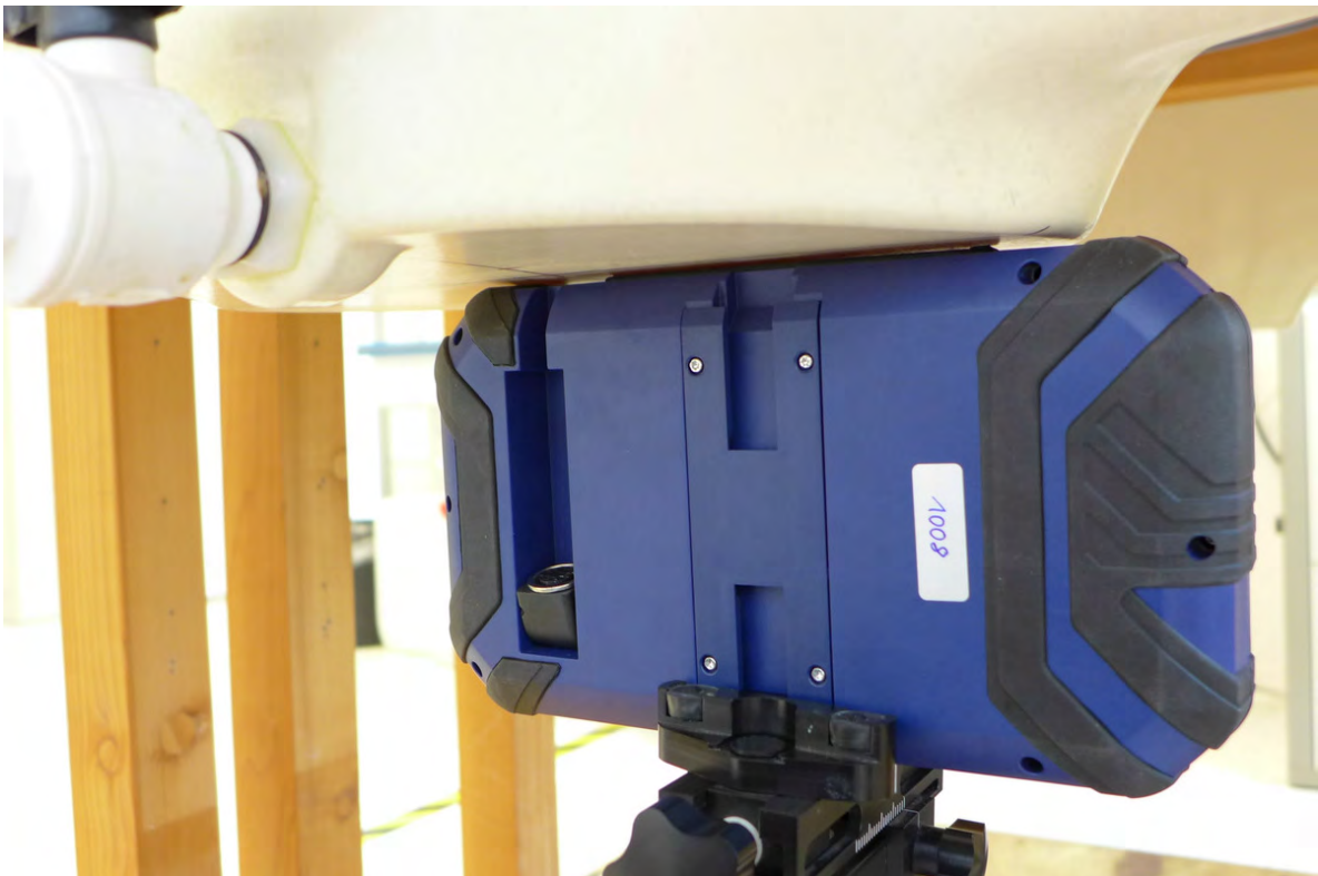
Pic. 9: Test position bottom side of DUT towards the phantom, 0 mm gap.
