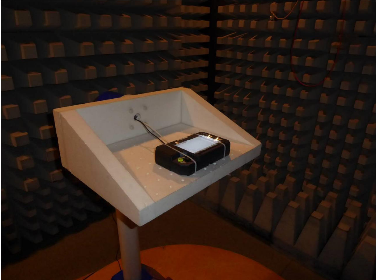
180488_radio_01.JPG: Test setup – radiated test in anechoic chamber
