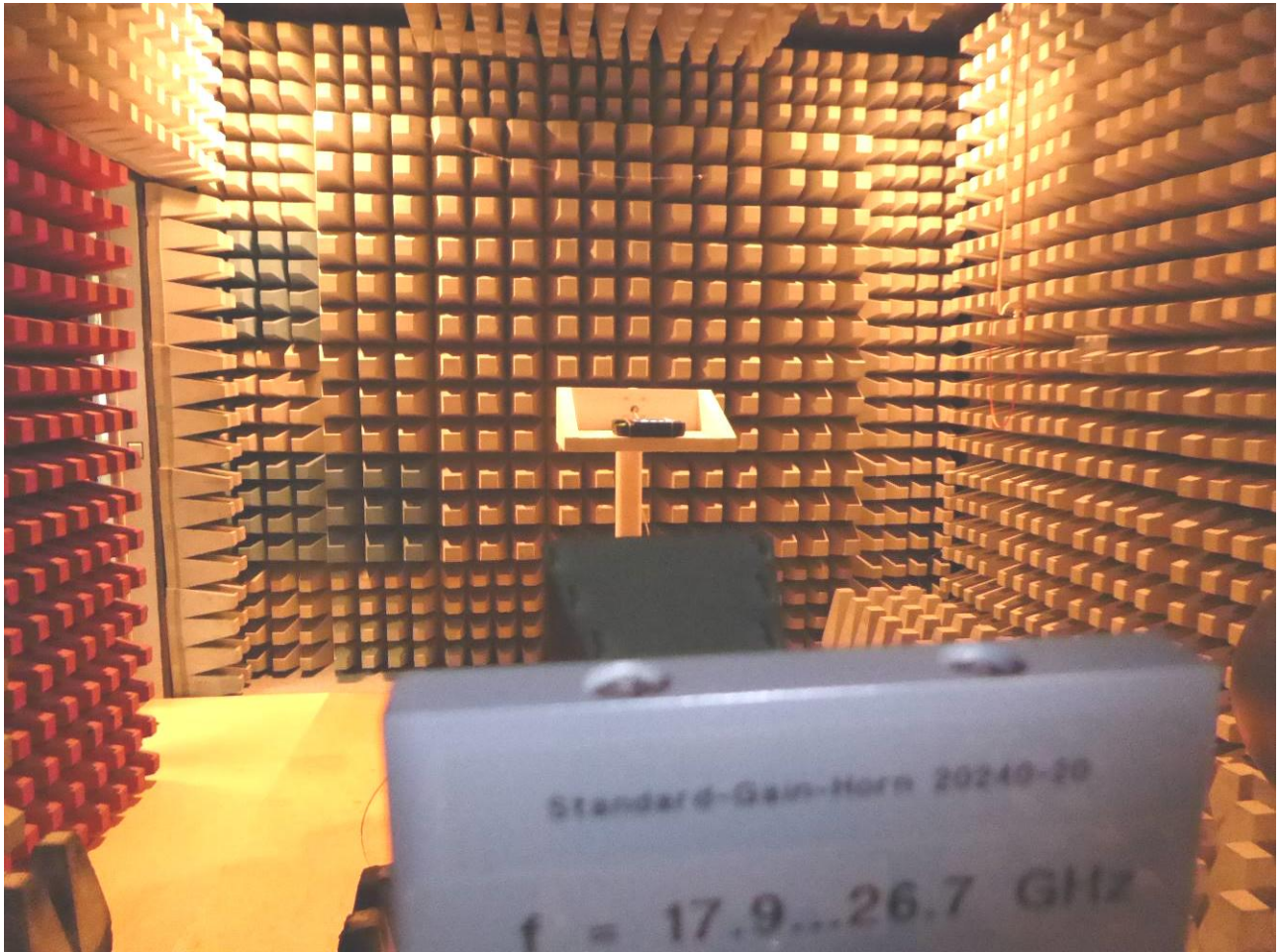
180488_radio_06.JPG: Test setup – radiated test in anechoic chamber
