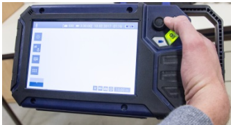
Fig. 13: With the handle pulled out it is possible to hold and operate the monitor with one hand.
