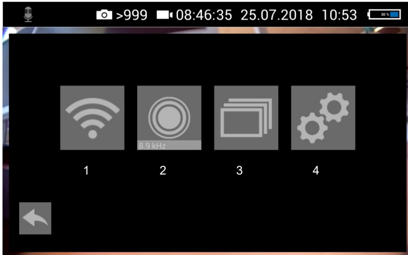
Fig. 29: System menu with submenus WLAN (1), Locator detection (2), Image and video gallery (3) and settings (4)
