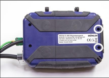
Fig. 50: Bottom of the device - Open the cover by loosening the cross-head screws .
