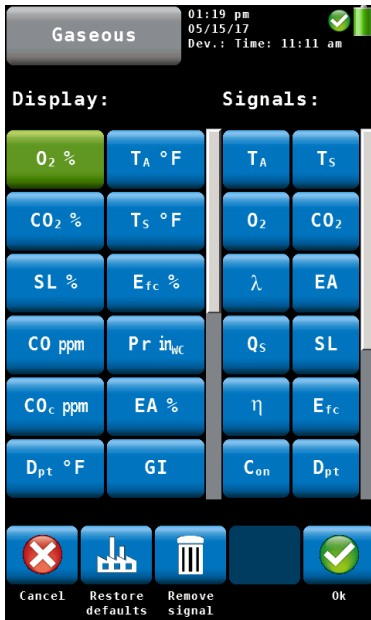
Fig. 38: Configuration of the readings segment.
