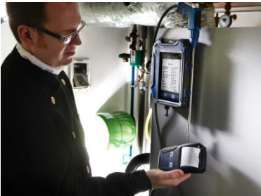
Fig. 23: Printing the readings of the Wohler A 450 on the Thermoprinter Wohler TD 100.
