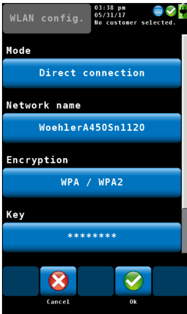
Fig. 35: WLAN configuration – Direct connection
