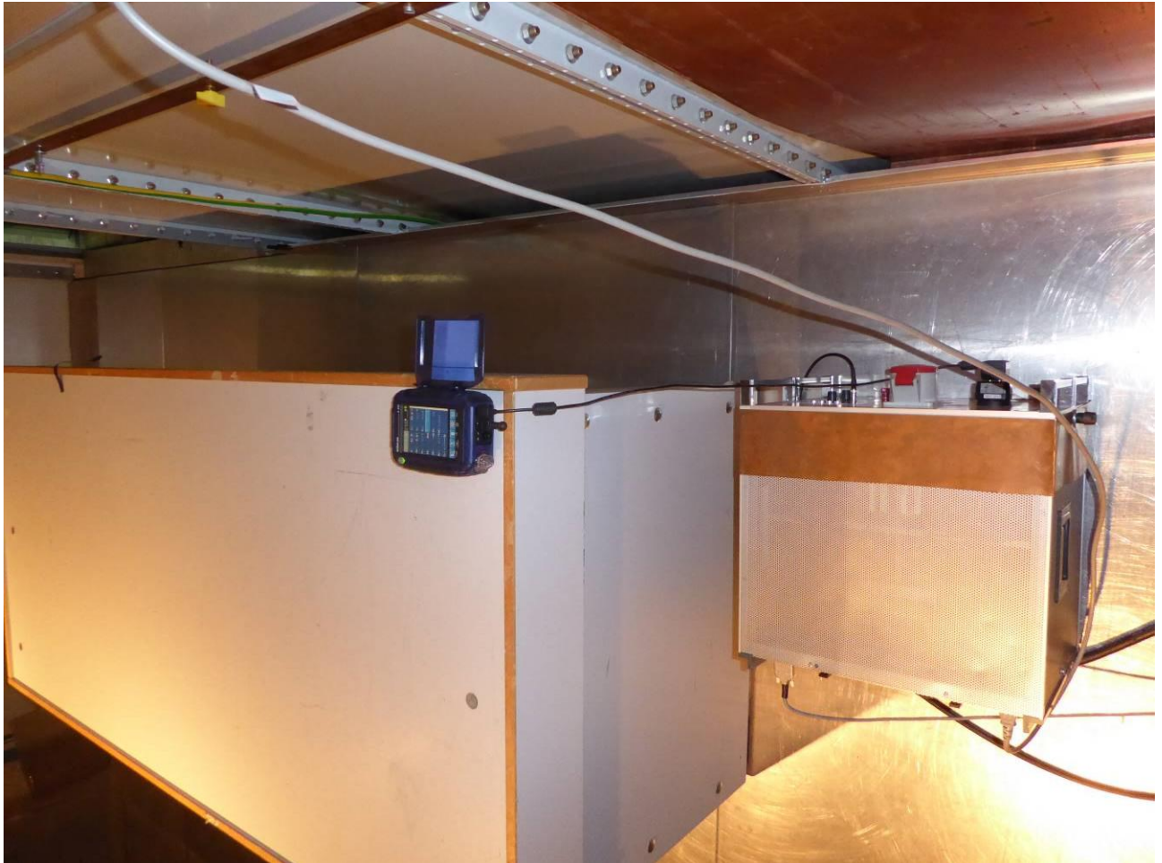
170475_09: Test setup – conducted emissions on power supply lines
