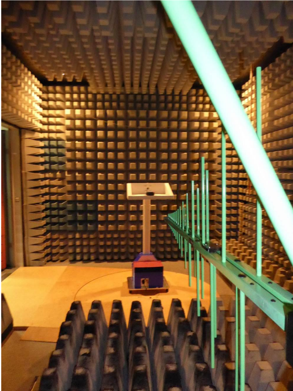
170475_03.JPG: Test setup – radiated test in anechoic chamber
