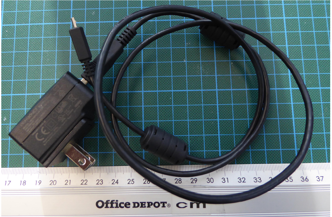
170475eut5d.jpg: Power supply cable
