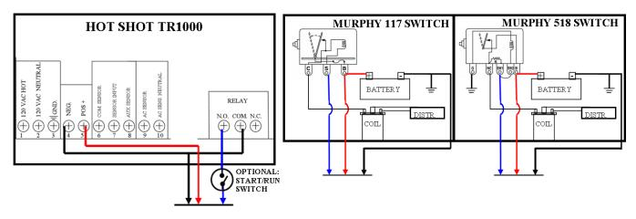
PUMP START: IF USING A START/RUN SWITCH FLIP IT TO START. POWER UP THE HOT SHOT AND START THE ENGINE AT THE PUMP. WHEN THE PIVOT IS PRESSURED UP IT'S HOT SHOT WILLTRANSMITT A RELAY ON COMMAND TO THE HOT SHOT AT THE PUMP. WHEN A RELAY ON COMMAND IS RECEIVED THE HOT SHOT WILL CLOSE ITS N.O. TO COM CONTACTS AND LIGHT UP THE RELAY LED. THIS WILL REMOVE THE GROUND FROM THE MURPHY ALLOWING THE ENGINE TO STAY RUNNING. IF USING A START/RUN SWITCH FLIP IT TO RUN.
