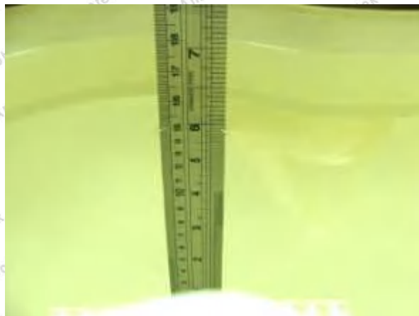
Photo of Liquid Height for Head SAR
