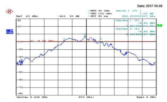
Modulation Standard: GFSK (1Mbps) Channel: 39
