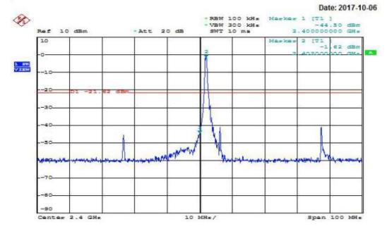
Modulation Standard: GFSK (1Mbps) Channel: 39
