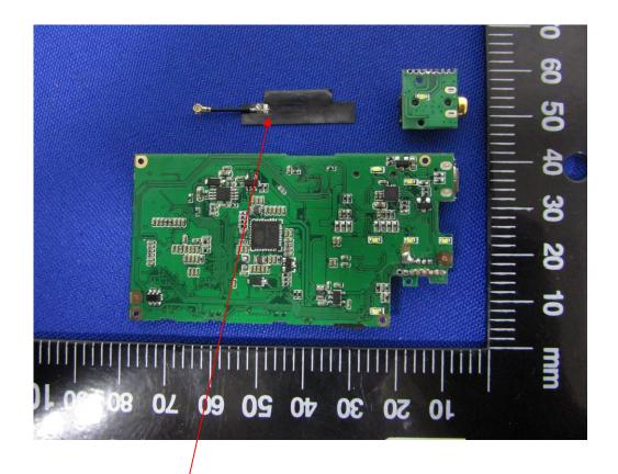
This is a Integral antenna, antenna gain is -0.3dBi.
