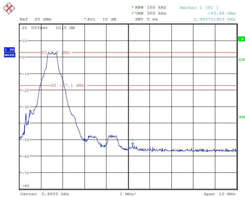
**EDR ( $\pi/4$ -DQPSK): Band Edge-Left Side****Hopping**
