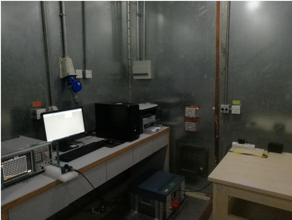
FCC RADIATED EMISSION TEST SETUP
