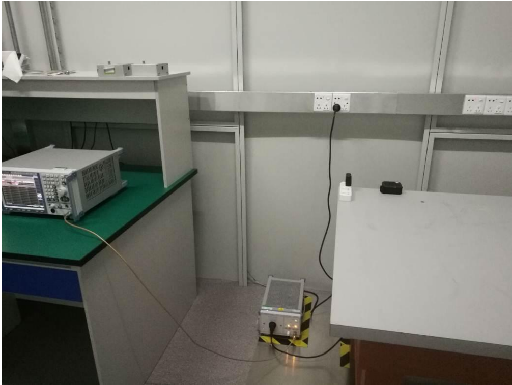
FCC RADIATED EMISSION TEST SETUP
