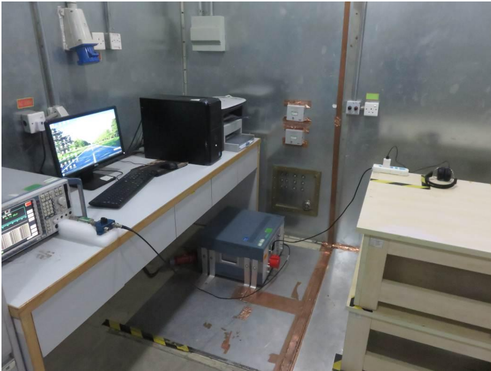
FCC RADIATED EMISSION TEST SETUP
