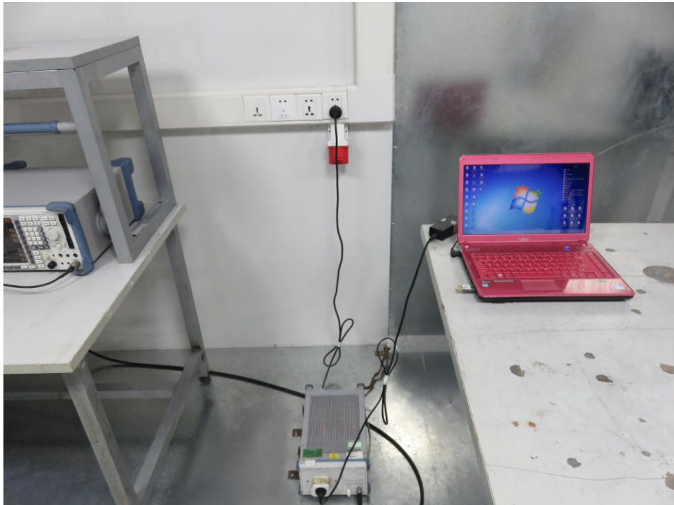
Photo of Conducted Emission Test
