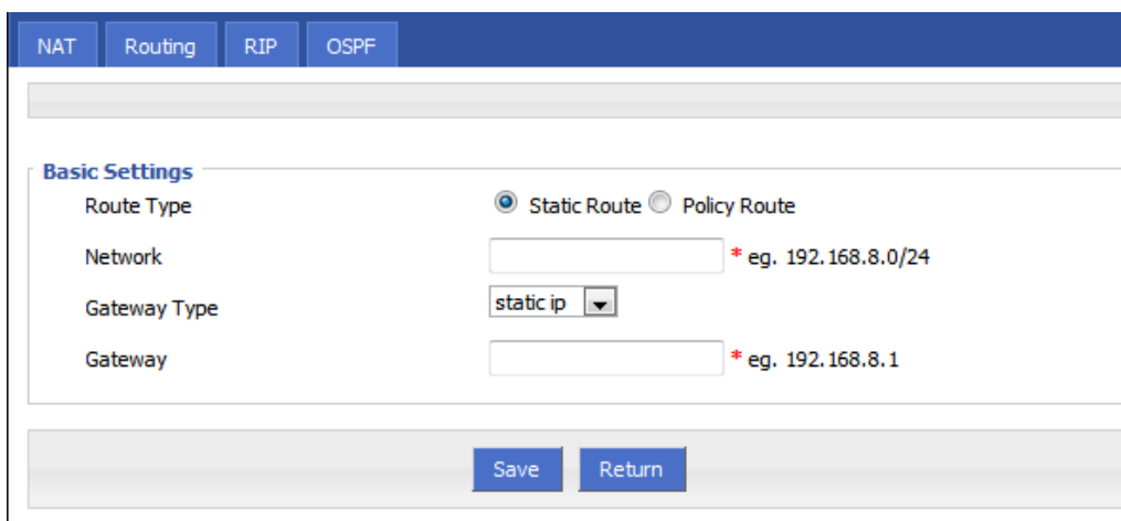
Figure 5-35 Static Routing Interface
