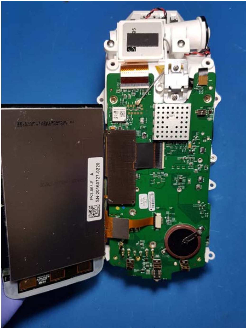
Top Side View with LCD lifted and LCD frame removed
