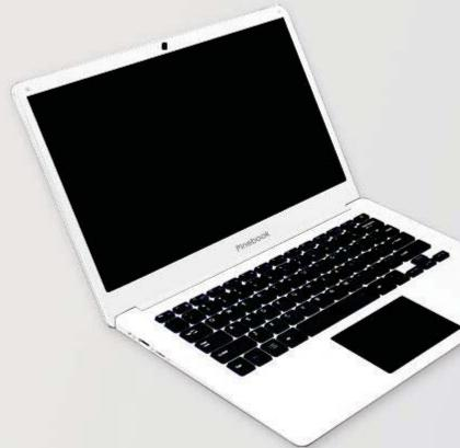
A 14" Notebook powered by Quad-Core ARM Cortex A53 64-Bit Processor
