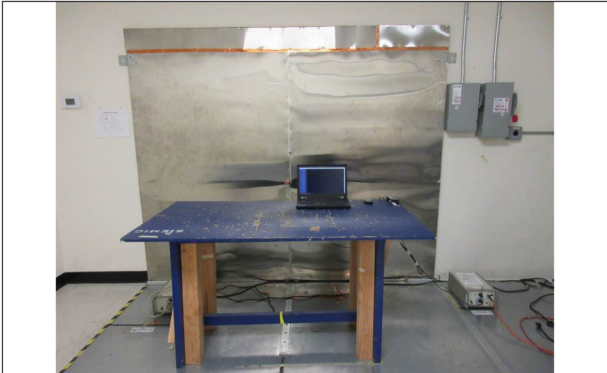
Conducted Emission Test Front View
