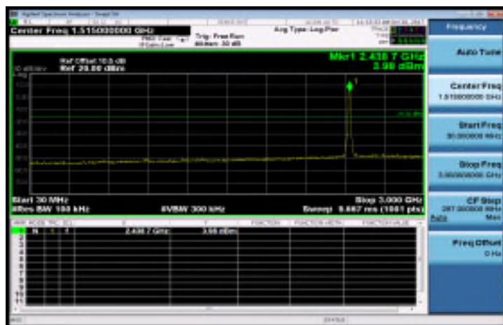
802.11n_HT20: Spurious Emission Test Data CH-Mid
