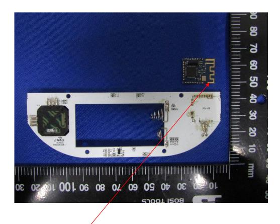
This is a BT antenna, antenna gain is 0dBi.
