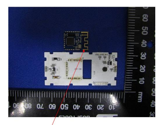
This is a PCB antenna, antenna gain is 0dBi.
