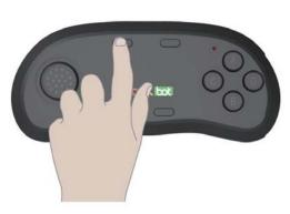
After the connection is successful, •••, • 0.5s flash, •always bright After the connection fails, ••• after, • 0.5s flash, • 1s slow flash
