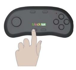
After the connection is successful,  $\bullet$  0.5s is flashing,  $\bullet$  light is on After the connection fails,  $\bullet$  0.5s flash,  $\bullet$  1s slow flash
