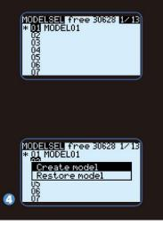
The Model Select menu allows the user to select the active model and allows the user to create, copy, move or delete a model. By selecting the "Create model" option, the new model guide (the script required by the guide is in the SD card) will be launched. The user will be leading through the basic control setup, if you choose not to use it, just press RTN Keys to manually set the model.
