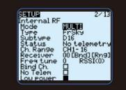
Status:Display the status of the multi-protocol module. (Normally it shows the firmware version of the multi-protocol module)
