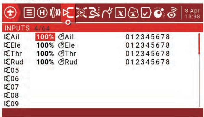
Since we only need two aileron and ELE inputs, we can delete the other two. Select the option you want to remove, long and hold the ENT key to pop up the edit window, then select the Delete option and press ENT.
