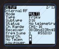
The default value of Frequene is "0". If the receiver does not bind, we can change the value to either +30 or -30 and try to bind again. If binding is still unsuccessful, continue to try higher and lower values in steps of plus or minus 30 until the bind succeeds.
