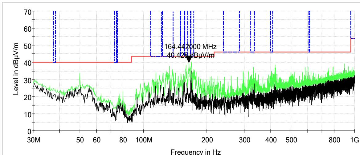
**Characterization Scan, 30 MHz to 1000 MHz, Horizontal, Channel 13**
