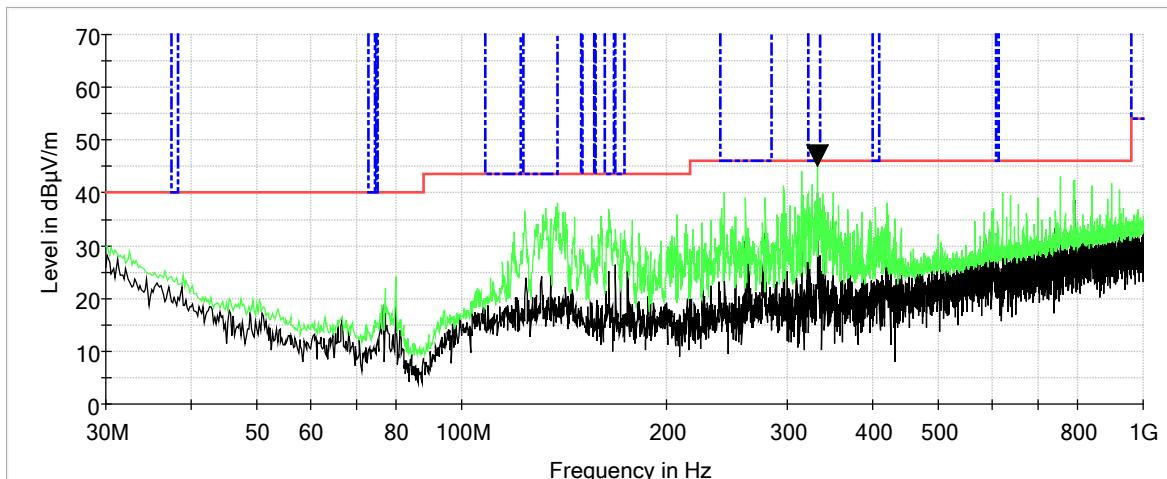
**Characterization Scan, 30 MHz to 1000 MHz, Vertical, Channel 13**
