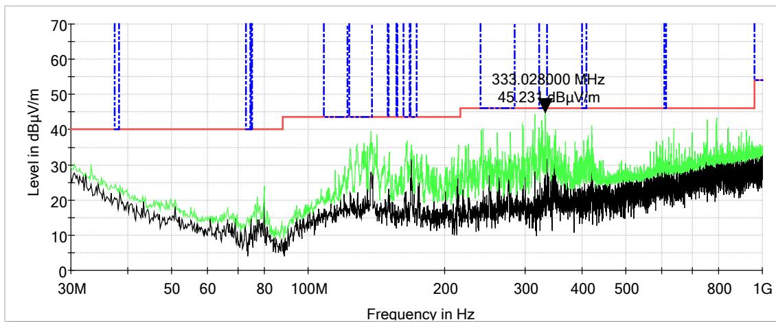
**Characterization Scan, 30 MHz to 1000 MHz, Vertical, Battery**
