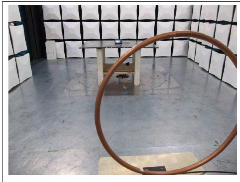
**Radiated Spurious Emission: Less Than 1 GHz**
