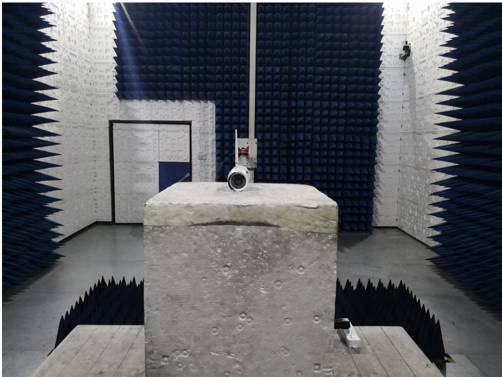
FCC RADIATED EMISSION TEST SETUP ABOVE 1GHZ
