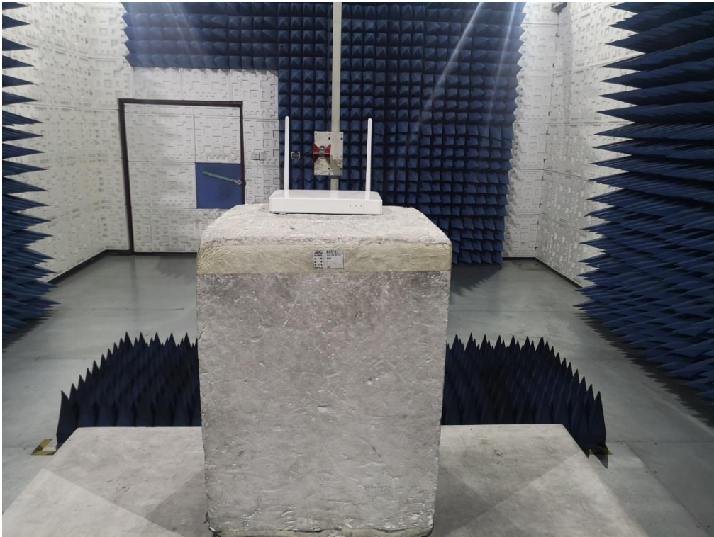
FCC RADIATED EMISSION TEST SETUP ABOVE 1GHZ
