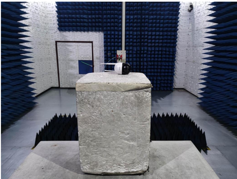
RADIATED EMISSION TEST SETUP ABOVE 1GHz
